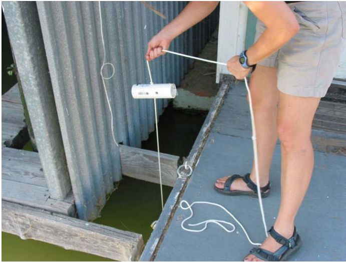
Figure 6. Zebra mussel sampling devices are composed of two PVC tubes stuffed with mesh and one plexiglass plate. Sample devices are placed near marina gas docks and boat ramps, locations where zebra mussels are most likely to be dislodged from boat hulls. Photos by C. Messer, DWR.
