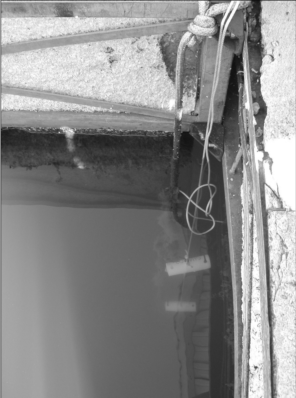
Figure 3.3. Zebra mussel substrate sampling device suspended in a boat slip at a marina.
