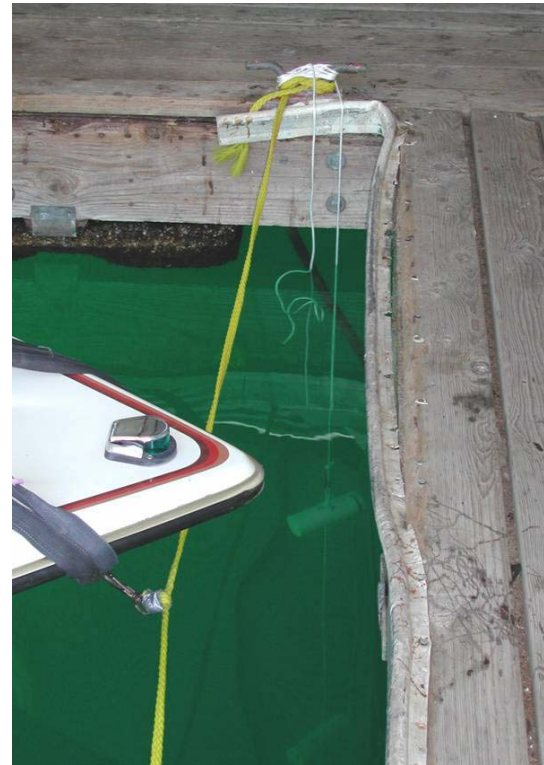
Figure 6. Zebra mussel sampling devices are composed of two PVC tubes stuffed with mesh and one plexiglass plate. Sample devices are placed near marina gas docks and boat ramps, locations where zebra mussels are most likely to be dislodged from boat hulls. Photos by C. Messer, DWR.
